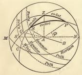
Thus, if A be any place, represented in the figure by a point at the center of the celestial sphere, the vertical line AZ determines the zenith Z. Let P be the celestial pole and N the north point of the horizon, then the angle PAN or the arc PN is the latitude of the place. In all questions relating to lati-
